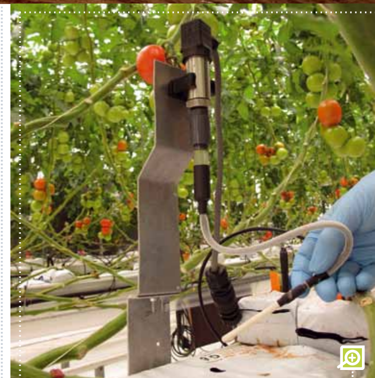
Figure 9: Installation of two tensiometers during a tomato cultivation trial on coco coir slabs. The pressure transducer is replaced by a digital recording system.
